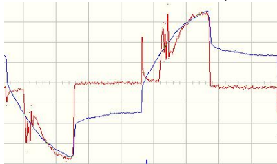
Reverse-phase 100% Dim Level Waveform Capture
