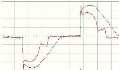
Forward-phase 100% Dim Level Waveform Capture
