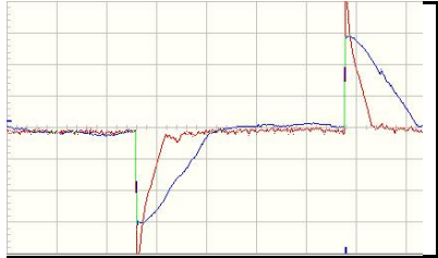
50% Dim Level Waveform Capture
