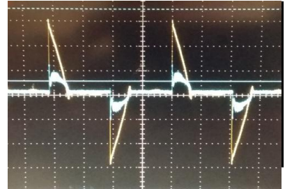
50% Dim Level Waveform Capture
