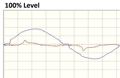
Voltage (blue) and Current (red) Wave
