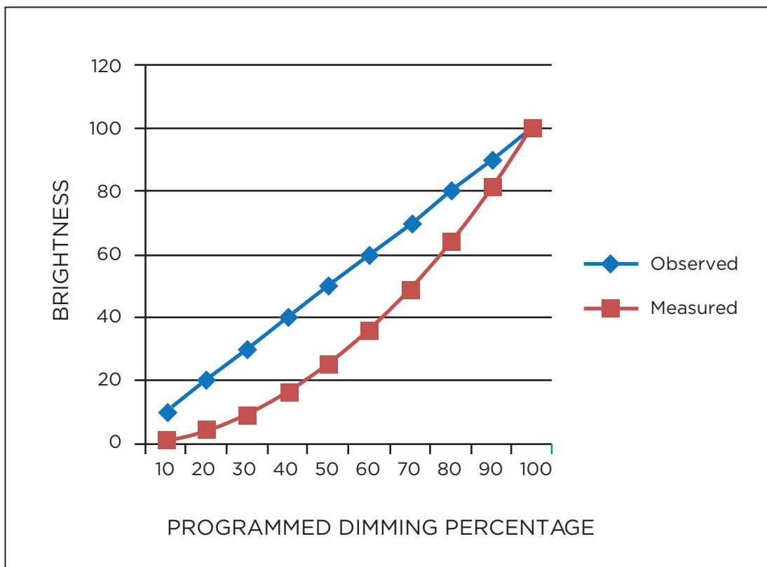
All Vantage InFusion-compatible line-voltage dimmers feature an ‘Adjust’ parameter designed to allow best fit to the ideal dimming curve. In the LED testing performed at Vantage, experimentation with the Adjust is performed to bring the curve as close as possible to the ideal.
