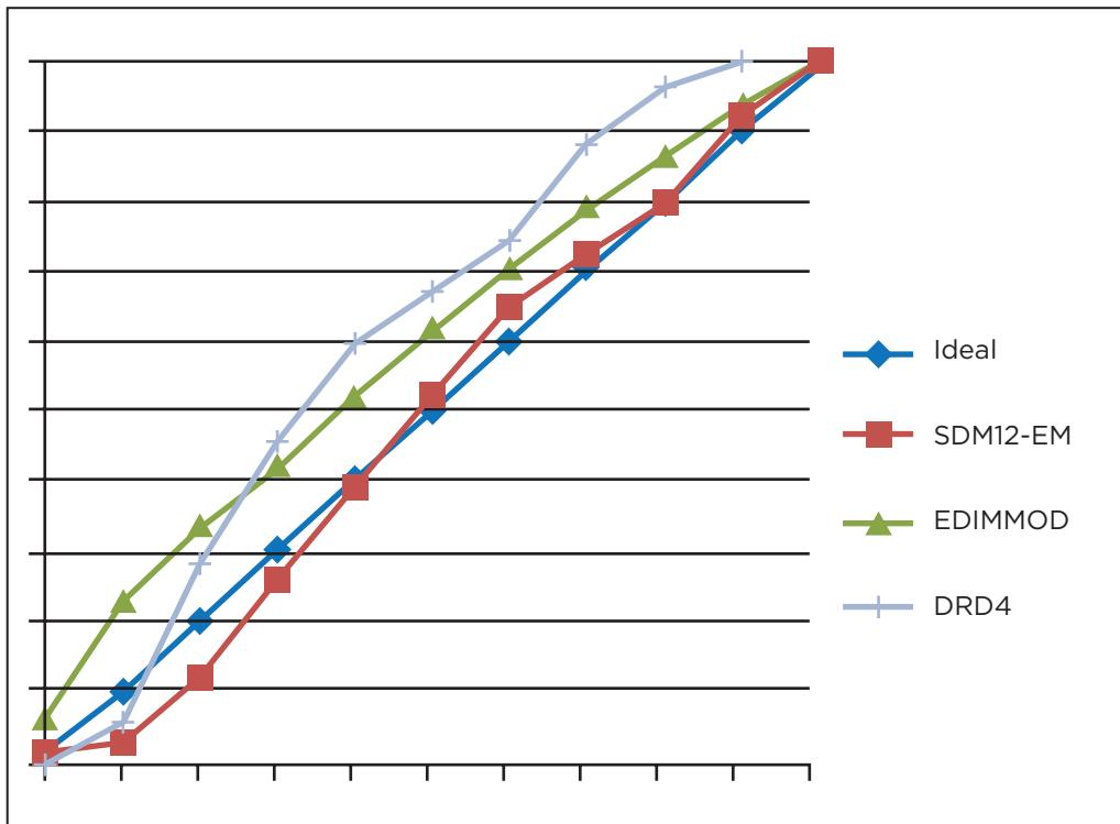
**The Power Profile** - Through InFusion Design Center software, custom power profiles can be defined and assigned to individual lighting loads. By applying a power profile that matches the best-fit power profile as determined through testing, we eliminate low-end anomalies and maximize dimming linearity. The adjustable parameters of the power profile are:
